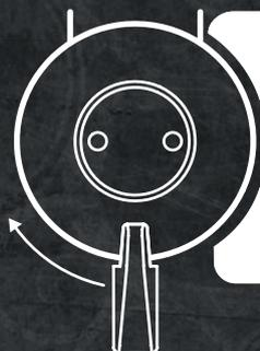
By controlling the flow of water and pressure mechanically via an internal valve, you can reproduce the superior cup quality that has traditionally been attained with "lever" machines. Manual pre-infusion allows you to bring out different flavor components which affect the balance and body of the shot, and produce a rounder, softer espresso that highlights brightness, sweetness and delicate notes.
